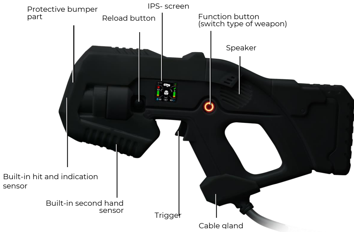
The main elements of the blaster
