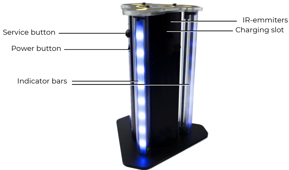
External view of Smart DB
