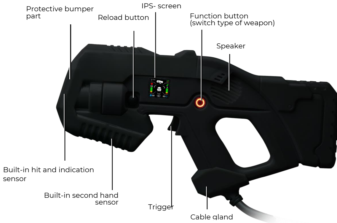
The main elements of the blaster
