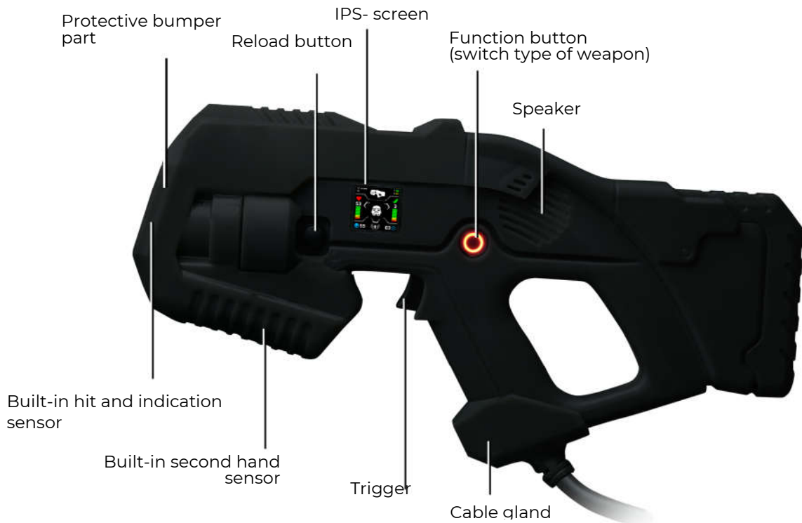
The main elements of the blaster
