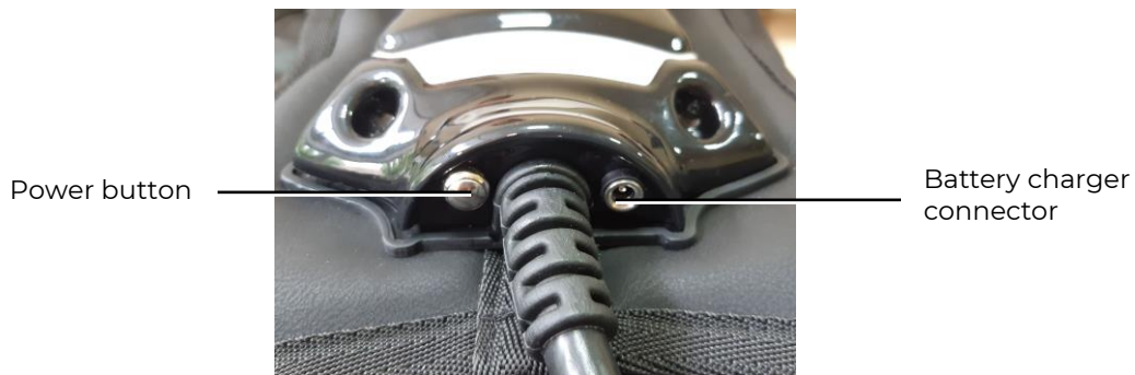
External elements of control unit
