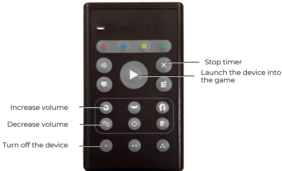
The buttons on the Remote Control for controlling the laser tag bomb without a server
