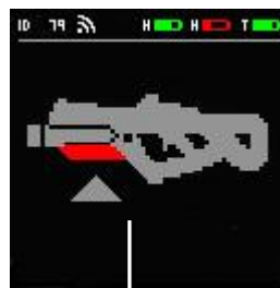
Two-hand absence sensor tripped
