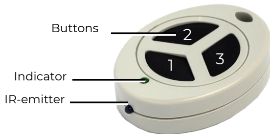
The external view of the remote control and the numbering of buttons
