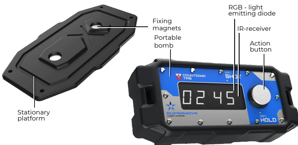
Components of the Laser Tag Bomb
